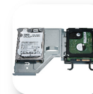
Tool-less 2.5" HDD and ODD mounting
